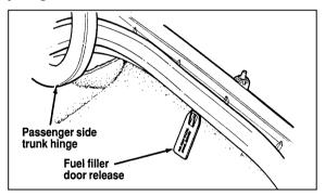
The fuel filler door manual release — located inside the trunk
